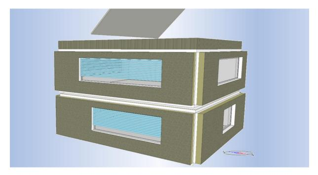
Figure 4: Single house configuration with expected window to envelope ratio of 16,8%. West wall has no windows, northern windows have no shading. Upper ceiling has U-value 0,06 W/m2K, walls U-value varies with location (indicated in the table below).
