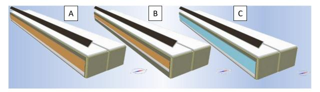
Figure 3: Glazing configurations. (A) fully glazed (100%); (B) partially glazed (70%, used also as label in charts as TGU/QGU 70%); (C) fully glazed with external venetians.
