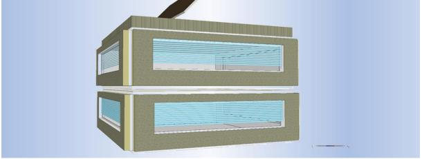
*Figure 5:* Single house configuration with expected window to envelope ratio of 23,7%. West wall has no windows, northern windows have no shading. Upper ceiling has U-value 0,06 W/m<sup>2</sup>K.
