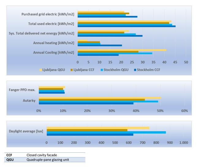
Quadruple-pane glazing solutions (without modulated external shades) for high volume to envelope ratios (business, office buildings) can be designed to offer comparable performance to CCF facades in all relevant (heating dominated) climates. This is mainly because reduced winter heat loss with pure quadruple panes offsets some weakness in cooling. With the PV attached this pronounced cooling is advantageous as PV works better in the summer.
