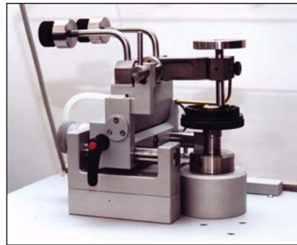
Figure 6. Pin-on-Disc wear tester (CSEM)
