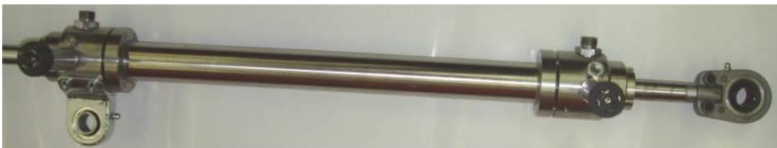
Figure 2: Specimen, a new water double-acting, double rod hydraulic cylinder
