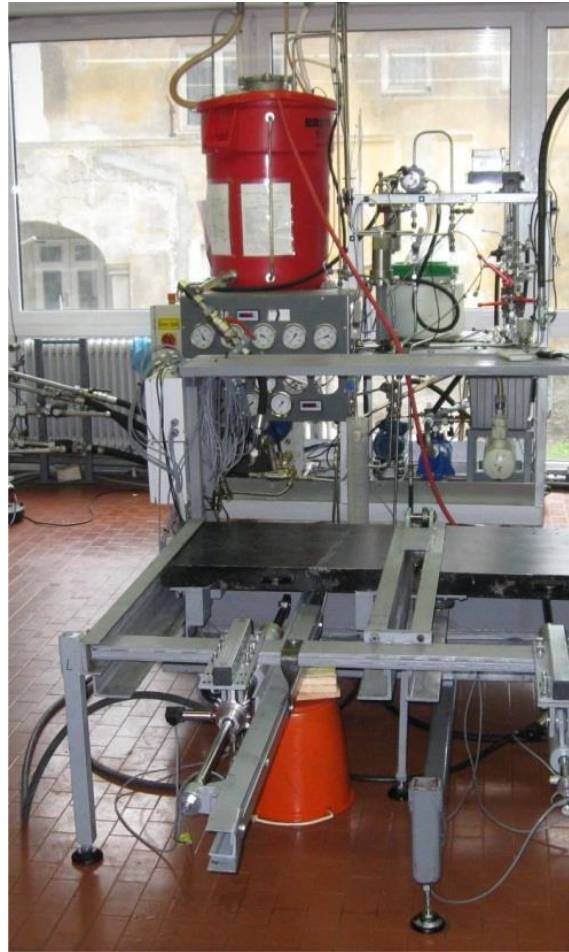
Figure 1: a. Simplified hydraulic circuit for the water hydraulic test rig, b. Photo of water hydraulic test rig
