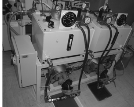
Figure 2: A hydraulic piston pump test rig with two separate testing systems (circuits).
