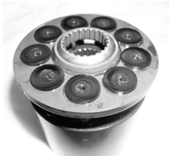
Figure 1: Assembly of pistons with DLC-coated shoes, inserted in pump cylinder block.
