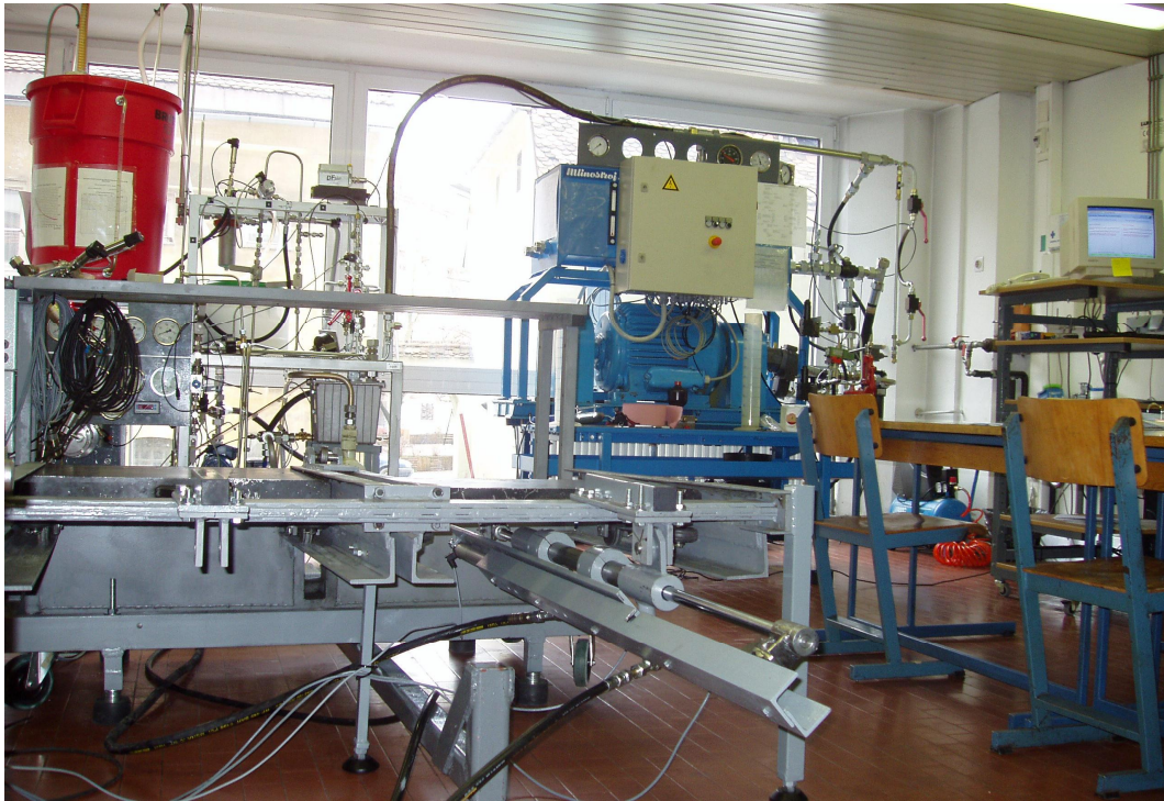
Figure 2. Double, water and oil hydraulic test rig
