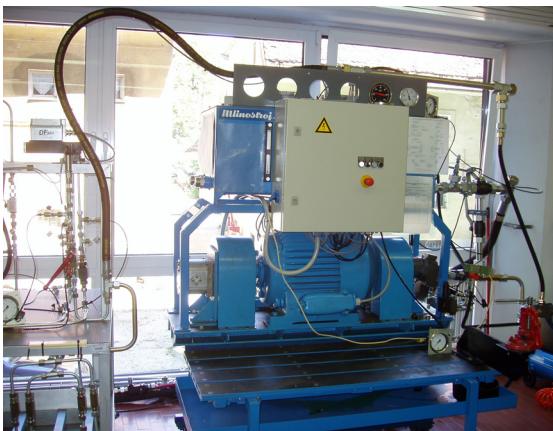
Fig. 3. Oil power-control part of the test rig
