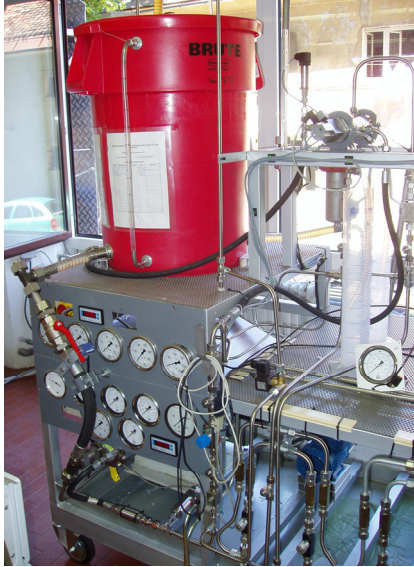
Fig. 2. Water power-control part of the test rig
