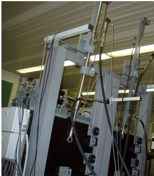
Fig. 6. Water (on the left) and oil (on the right) hydraulic cylinder with load masses
