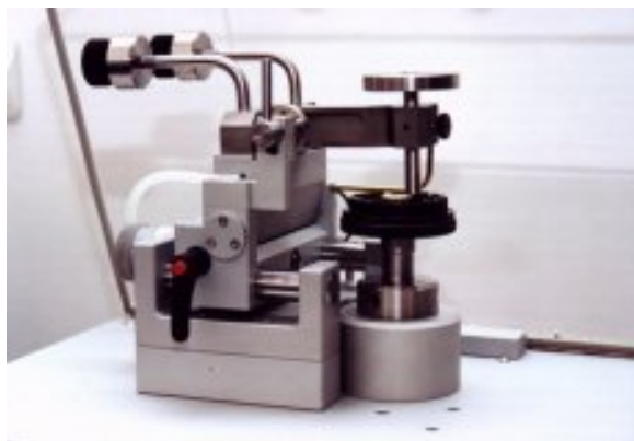
Figure 6: Pin-on-Disc wear tester (CSEM)
