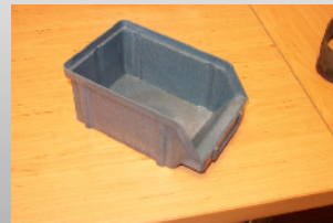
Screw box made from PP-wood composite
