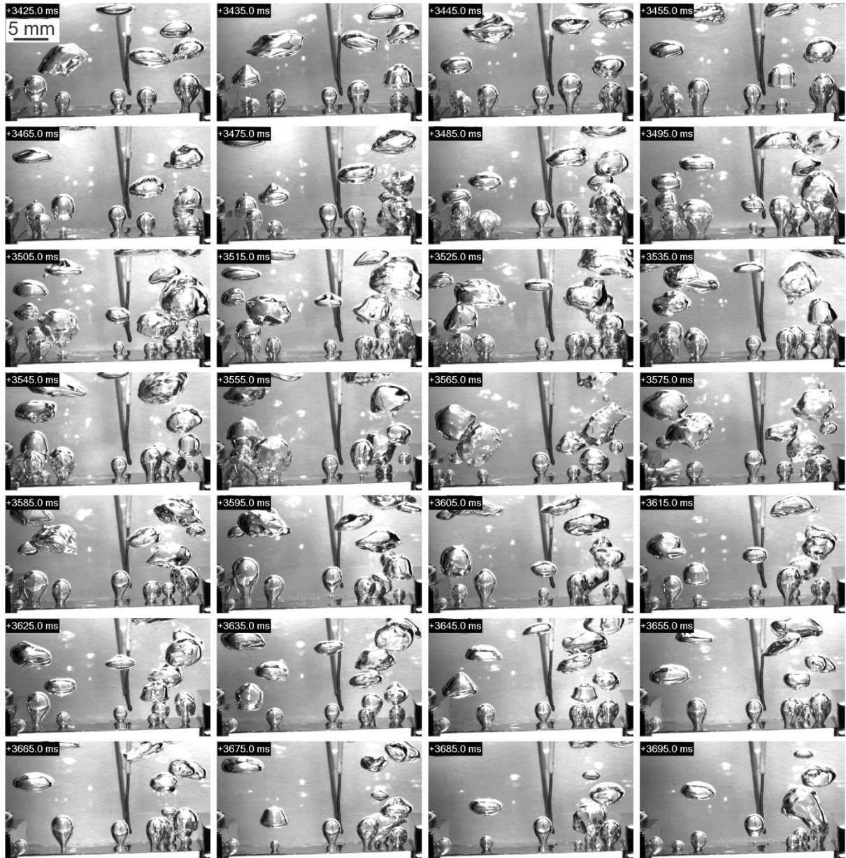
Supplementary Figure 5. Consecutive video images of saturated nucleate boiling of water on non-processed stainless steel foil (SS) at 50 \text{ kW m}^{-2} . Time step between images is 10 ms.
