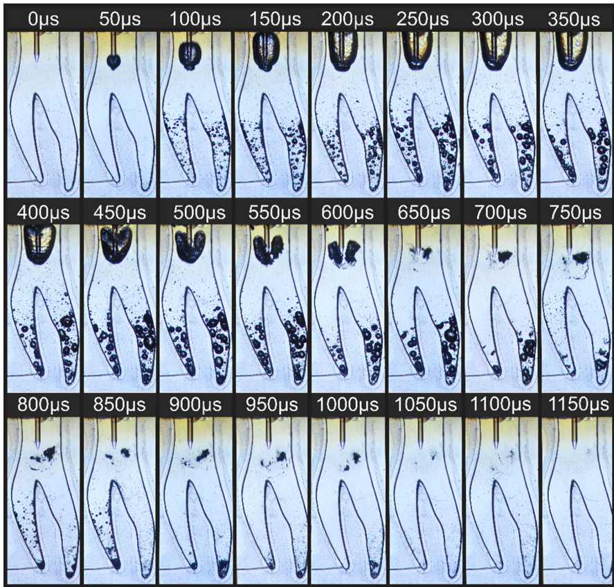
Fig. 2 The series of images shows the life cycle of a laser-induced vapor bubble. Because light of wavelength 2.94\text{ }\mu\text{m} is strongly absorbed in water, a very thin layer of water next to the FT is heated up in a very short amount of time beyond its boiling point. This leads to explosive boiling and a rapid expansion of the cavitation bubble ( 0\text{ }\mu\text{s} to 300\text{ }\mu\text{s} ). This process continues until the pressure inside the bubble is equal to the outside pressure, at which point the bubble starts collapsing ( 350\text{ }\mu\text{s} ). After the initial collapse of the bubble ( 700\text{ }\mu\text{s} ), additional oscillations can occur
