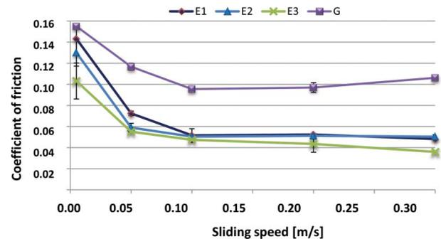
Figure 6. Influence of sliding speed and spacing between the dimples on the coefficient of friction in a lubricated sliding contact.
