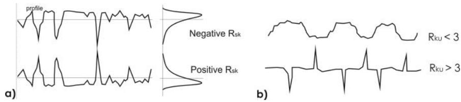
**Figure 1.** Schematic presentation of roughness profiles for (a) positive and negative skewness ( $R_{sk}$ ) and (b) kurtosis lower and higher than 3.
