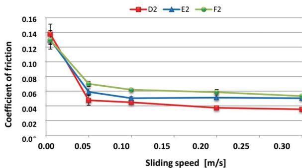
**Figure 7.** Influence of sliding speed and dimple depth on the coefficient of friction in a lubricated sliding contact.
