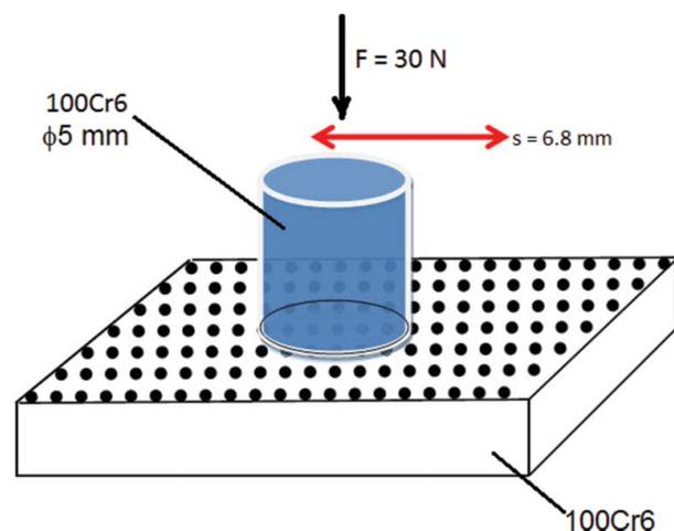
**Figure 4.** Schematic illustration of the contact between the pin and textured sample.
