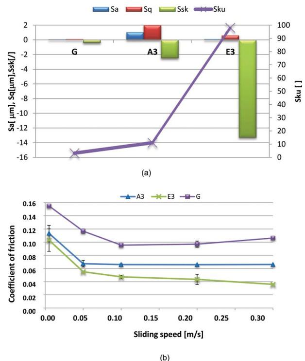
**Figure 8.** Effect of texture shape (G, ground; A3, channels; E3, dimples) on (a) the roughness parameters and (b) the coefficient of friction at different sliding speeds in a lubricated sliding contact.
