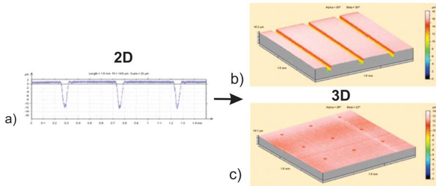
**Figure 2.** Transformation of the 2D profile (a) into 3D space; (b) in one ( $y$ ) direction and (c) in two ( $x$ - $y$ ) directions.
